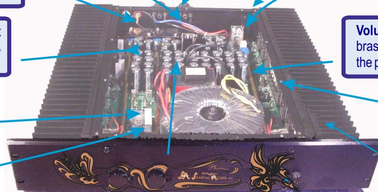
**Undiminished bass** from directly coupling the amp output to the speaker without capacitors. DC protection relays protect the speakers in case anything should ever happen to the amp.
